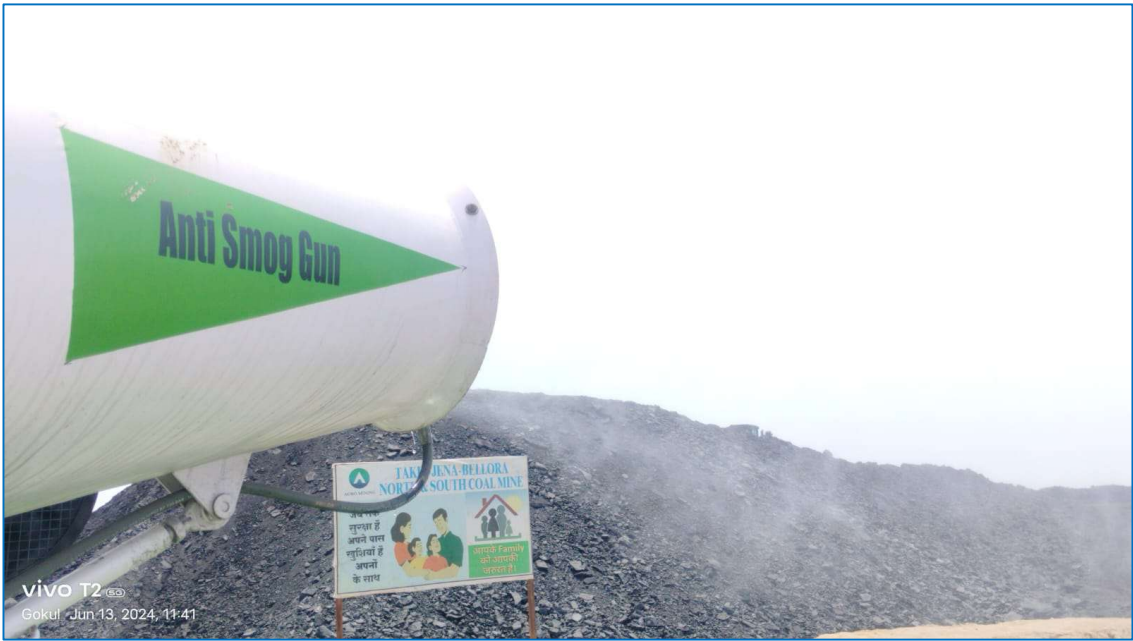
Fog Canon arranged at Coal Stock Area
