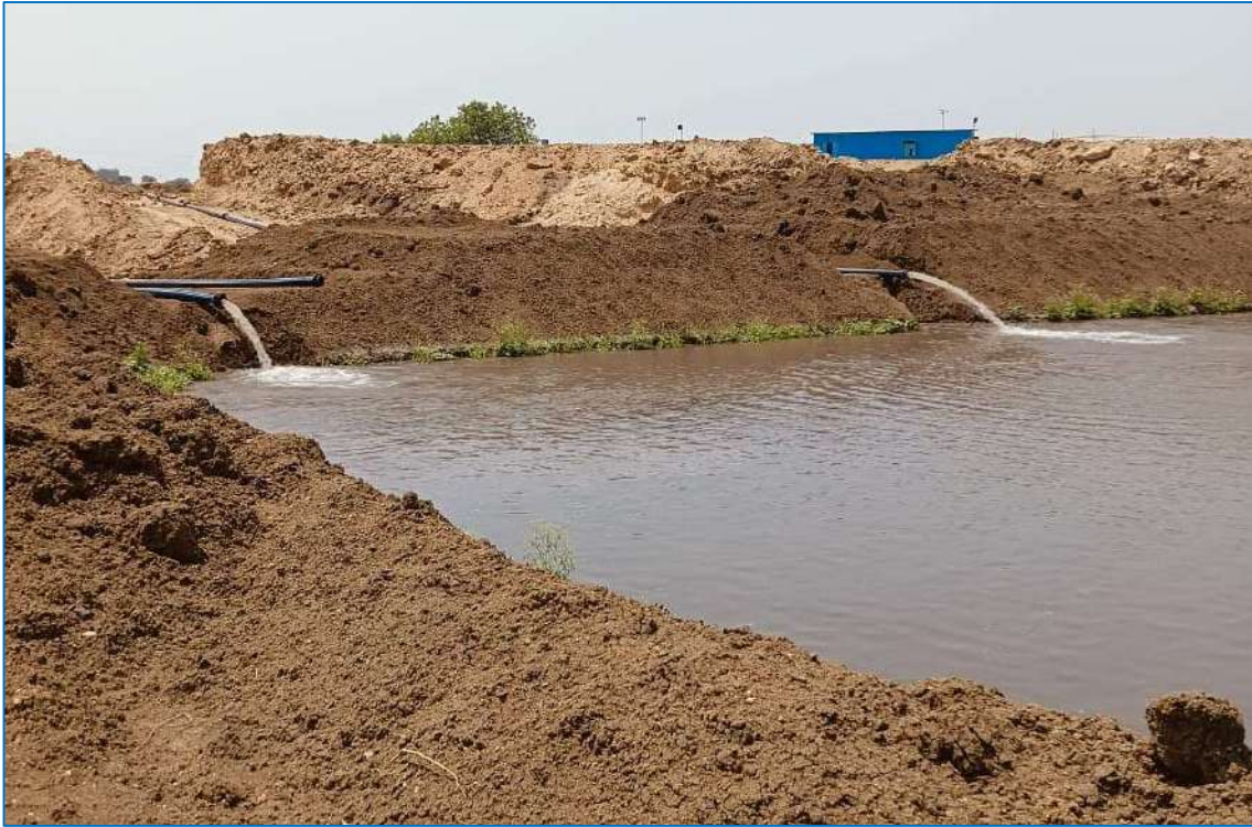
Mine seepage water pumping into sedimentation tanks
